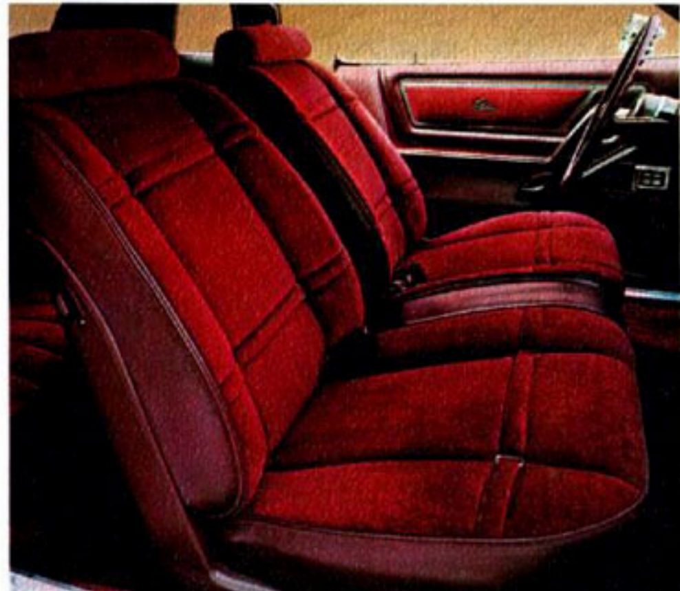
Standard "Verdi" velour cloth bench seat with vinyl accents and folding center armrest.
