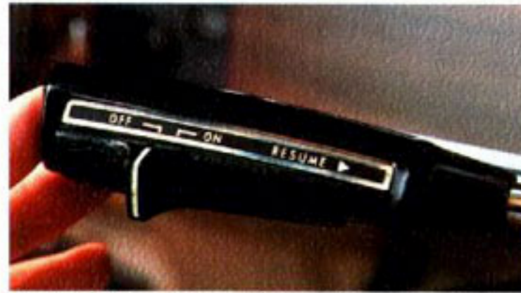
Optional Automatic Speed Control lets you select and hold a steady speed for driver ease and, possibly, improved mileage in highway driving.
